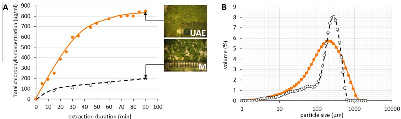
**Fig. 2.** Effect of power ultrasound on spinach leaves. (A: Comparison of chlorophyll extraction kinetics for UAE, US probe 20 kHz (●) and for maceration (M, ○); B: Comparison of particle size repartition (below 1 mm) of spinach residue for UAE (●) and for maceration (○)).
