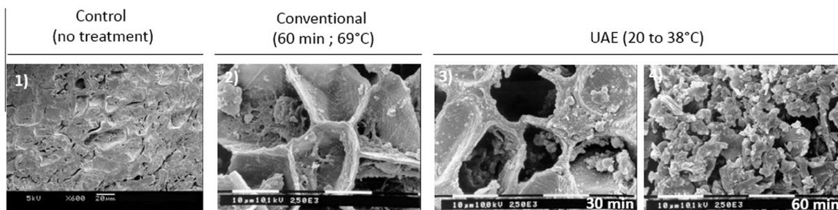
**Fig. 7.** Effect of power ultrasound on carvi seeds. (SEM microscopy for untreated seeds (1), seeds after conventional extraction (2) and UAE: US probe, 20 kHz after 30 min, (3) and after 60 min, (4)).
