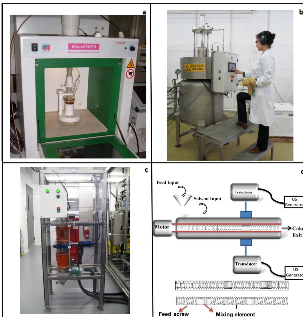
Fig. 10. Combined innovative extraction techniques ((a) ultrasound-microwave, (b) ultrasound – DIC, (c) ultrasound-SFE, (d) ultrasound-extrusion).
