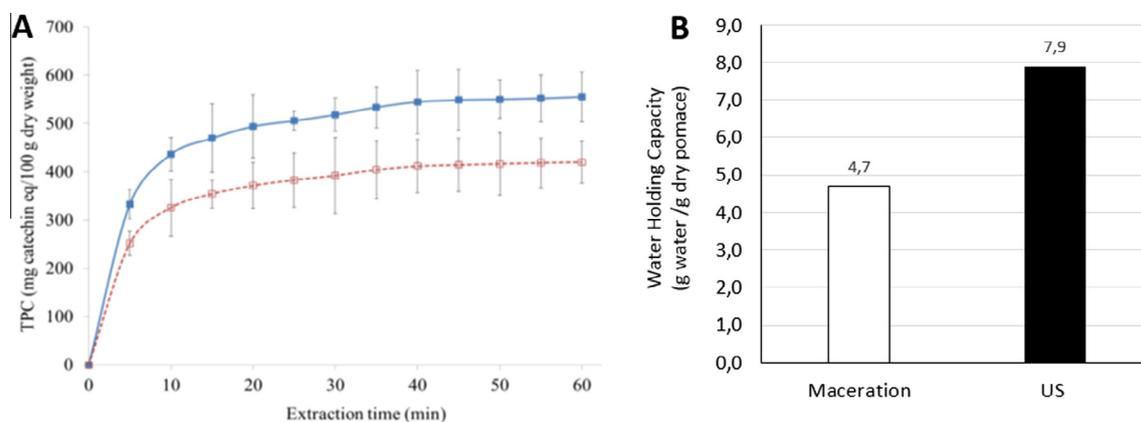
**Fig. 4.** Ultrasonic capillary effect induced by high power ultrasound on apple pomace. (A: Comparison of total polyphenol extraction (TPC) by maceration under agitation (●) and by ultrasound (ultrasound reactor 1 L, 25 kHz, ambient temperature) (●); B: Comparison of Water Holding Capacity of apple pomace after 10 min, for maceration under agitation and ultrasound (US probe, 20 kHz, ambient temperature)).
