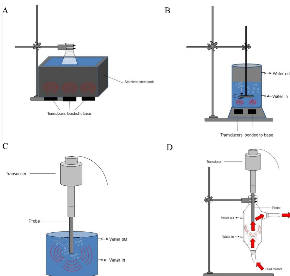
Fig. 8. Commonly used ultrasonic systems (A: Ultrasound bath, B: Ultrasound reactor with stirring, C: Ultrasound probe, D: Continuous sonication with ultrasound probe).
