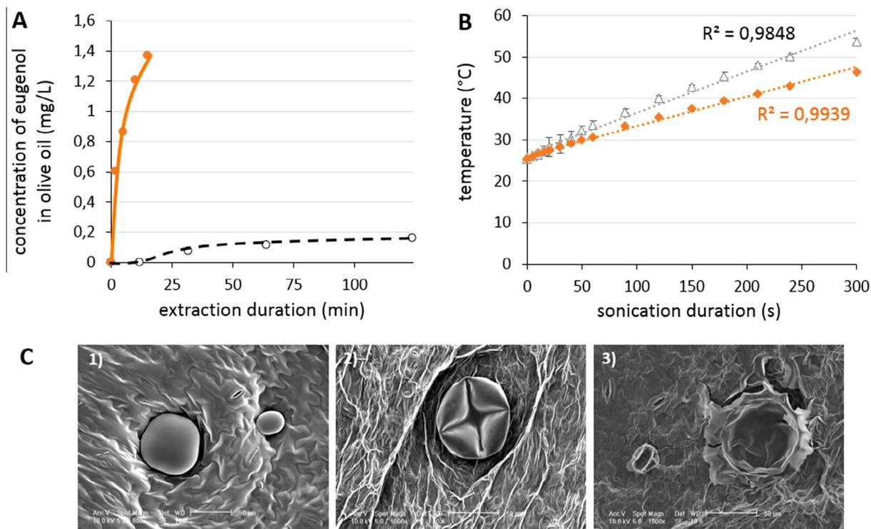
Fig. 6. Effect of power ultrasound on basil leaves. (A: Comparison of extraction kinetics of eugenol in olive oil for UAE, US reactor 25 kHz (●) and for maceration (○); B: US power dissipation during sonication for eugenol (◆) and olive oil (△); C: SEM microscopic observation of an essential oil gland, 1) control, 2) after maceration and 3) after UAE (US reactor 25 kHz).
