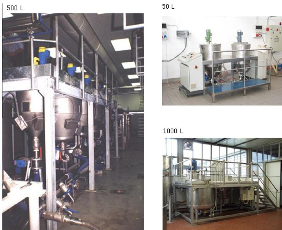
Fig. 12. Industrial ultrasonic batch equipments: 50, 500 and 1000 L (Reus – [www.etsreus.com](http://www.etsreus.com)).
